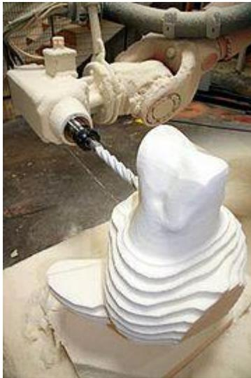
Robot machining part programmed using PowerMILL Robot Interface
