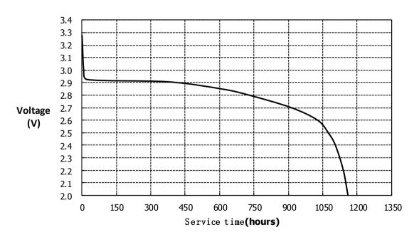
Discharge method:15K $\Omega$ , 24 hours/day EV 2.0V temperature of 20±2°C
