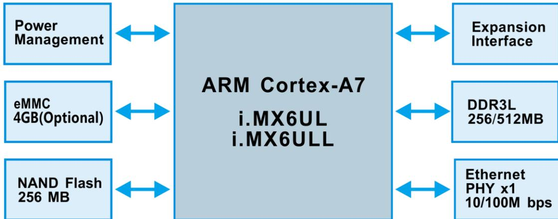
Figure 1-3 MYC-Y6ULX-V2 Function Block Diagram
