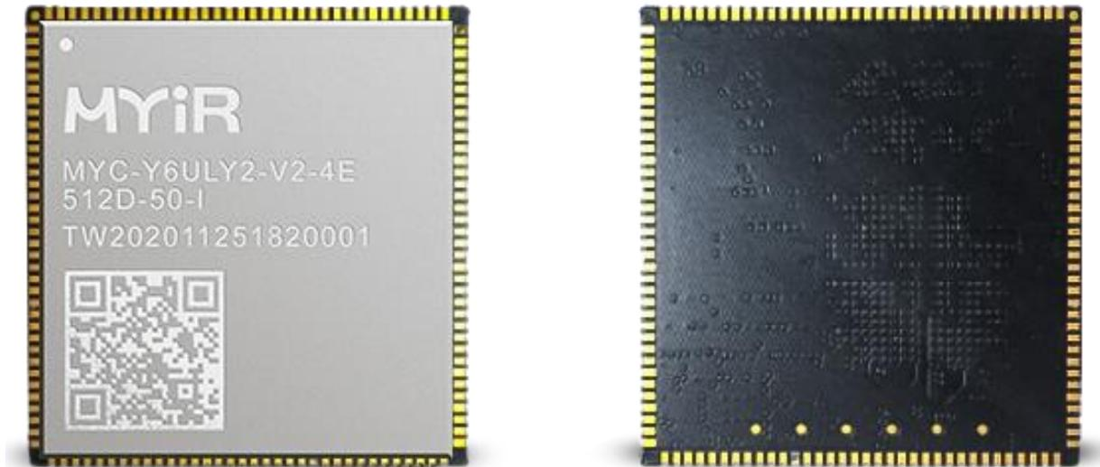
Figure 1-1 MYC-Y6ULX-V2 CPU Module (delivered with shield cover)
