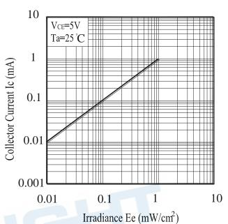
Fig.3 Collector Current vs.
