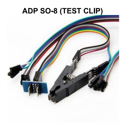
The **EE100 ISP SO8 Test Clip** is used to connect the ISP EE100 programmer to the Main EEPROM soldered on board offering the possibility to update directly the EEPROM content if no ISP connector is mounted on board. The ISP updating method must only been used if supported by your application or controller.
