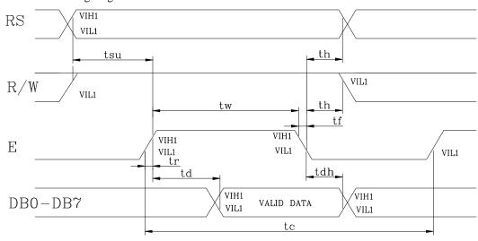
Write cycle (Ta=25 °C, VDD=5.0V)
