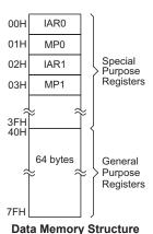
Note: Most of the Data Memory bits can be directly manipulated using the "SET [m].i" and "CLR [m].i" with the exception of a few dedicated bits. The Data Memory can also be accessed via the memory pointer registers.
