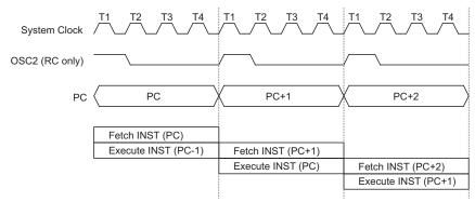
System Clocking and Pipelining
