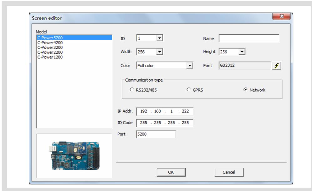
Figure6 “Screen editor” dialog box under network mode
