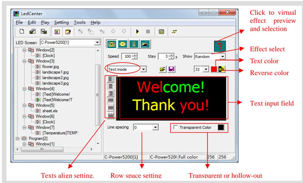
Figure21 Text program (text mode) edit interface
