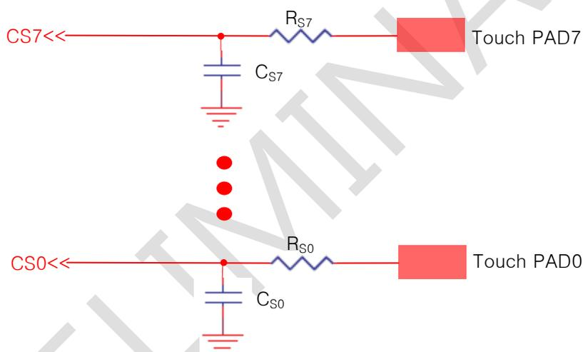
The ASRG08 has eight independent touch sensor input from CS0 to CS7. The internal touch decision process of each channel is separated from others. Therefore eight channel touch key board application can be designed by using only one ASRG08 without coupling problems.
