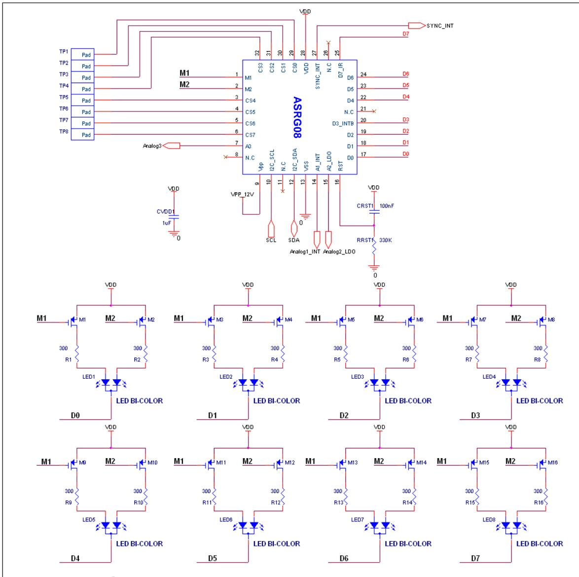
ASRG08-QD (32QFN) Application Example Circuit for 2-color LED
