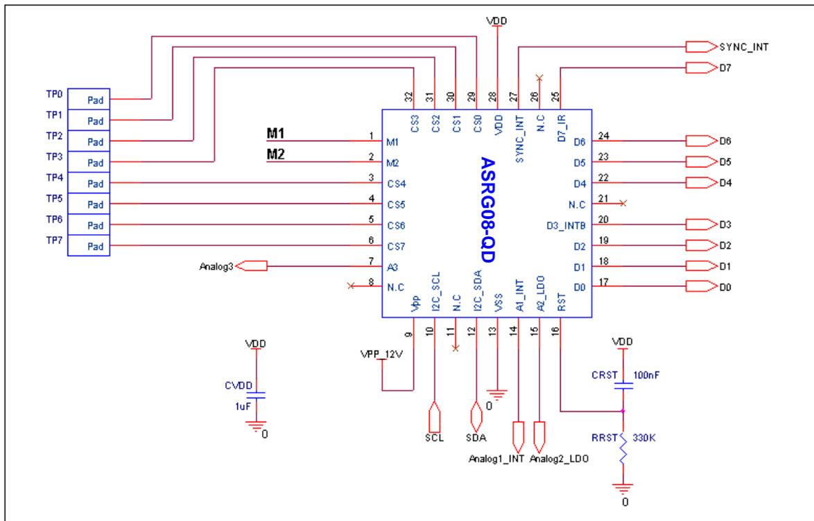
ASRG08-QD (32QFN) Application Example Circuit for parallel output
