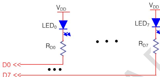
In the case of 2-color LED drive M1, M2 and D0~D7 must be equipped as below figure, and write the 'par\_output\_mode' bit of 'global\_ctrl2' register as '0' and the 'pwm\_sel' bit of 'global\_ctrl2' register as '1'. M1 and M2 have alternatively high and low pulse and the pulse duty is 50%. During M1 is high M2 is low, D0~D7 has 1pwm pulse of each D0~D7. During M1 is low M2 is high, D0~D7 has 2pwm pulse of each D0~D7.
