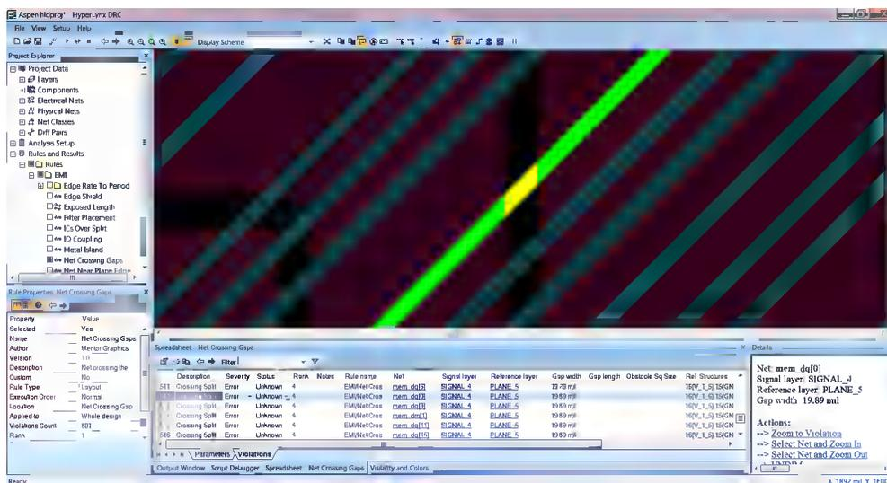
Design rule checks can be performed on boards for EMI/EMC issues, as well as signal integrity and power integrity issues. It is highly customizable, allowing users to create DRCs for any check they might otherwise perform manually.
