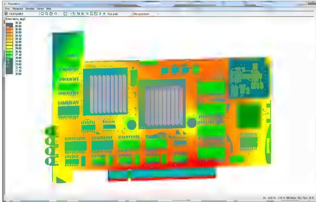
*Integrated thermal analysis allows engineers to detect potential heat problems without expensive prototyping.*
