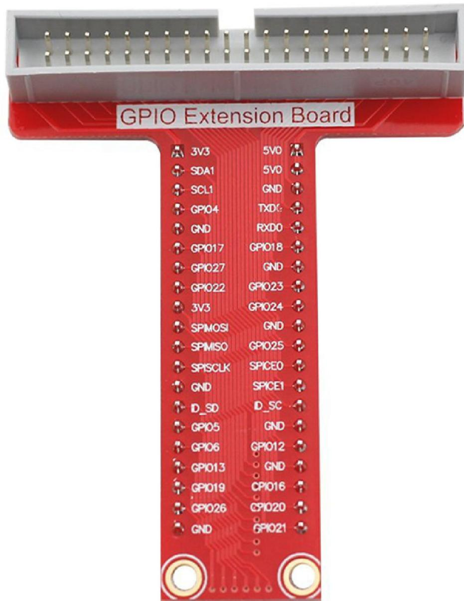
Connected with Raspberry Pi shown below, the principle is lead out the raspberry pi GPIO by GPIO cable to the GPIO pin extension board and extension board inserted into the breadboard, when you jump wire is inserted into the breadboard, equivalent inserted into the raspberry Pi GPIO.
