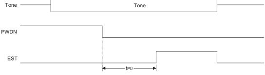
Figure 4. Power-up Timing
