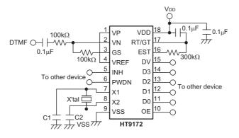
Note: X'tal = 3.579545MHz crystal C1 = C2  $\cong$  20pF X'tal = 3.58MHz ceramic resonator C1 = C2  $\cong$  39pF
