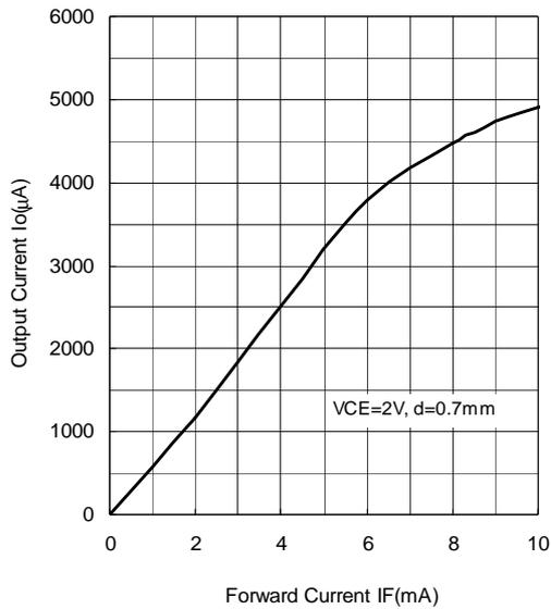
**Output Current vs. Forward Current
