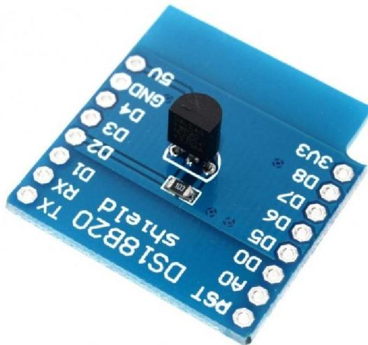
This shield is mounted with DS18B20 digital thermometer that provides 9-bit to 12-bit Celsius temperature measurements and has an alarm function with non-volatile user-programmable upper and lower trigger points. This sensor can be interfaced using 1-Wire bus that by definition requires only one data line and ground for communication. The pin used for this sensor is D2 pin of WeMos D1 Mini and Mini PRO, which rendered this shield to be not I2C compatible.
