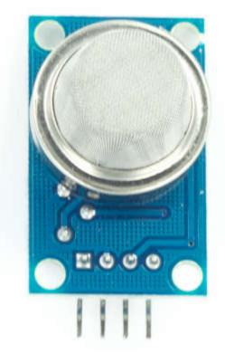
MQ-4 Module is used in gas leakage detecting equipment in family and industry, are suitable for detecting of CH4 ,Natural gas,LNG. Avoid the noise of alcohol and cooking fumes and cigarette smoke. The module gives out the concentration of the gases as a analog voltage equivalent to the concentration of the gases. The module also has a on-board comparator for comparing against a adjustable preset value and giving out a digital high or low.
